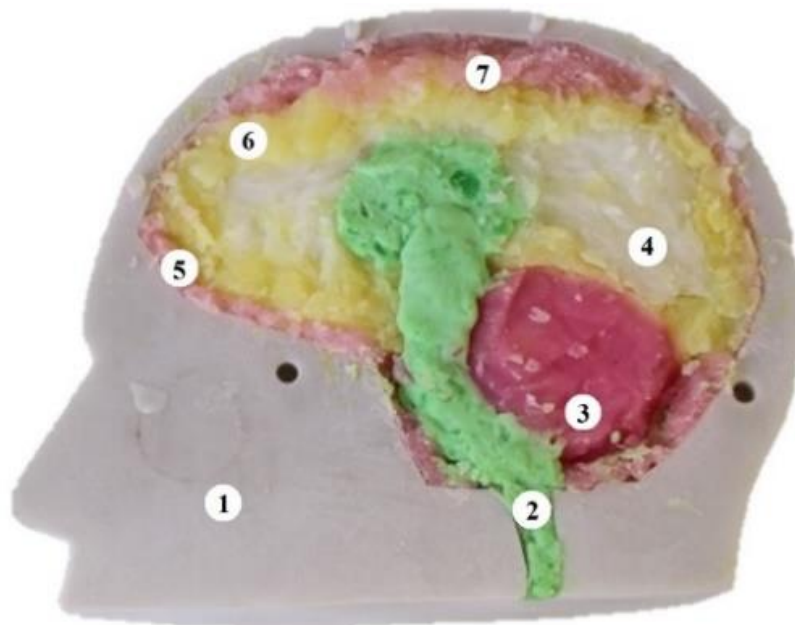
Fig. 3.8. Photograph of the internal structure of the fabricated 3D realistic human head [60]. 1) Exterior section, 2) spinal cord 3) cerebellum, 4) white matter, 5) Dura, 6) grey matter, 7) CSF.
