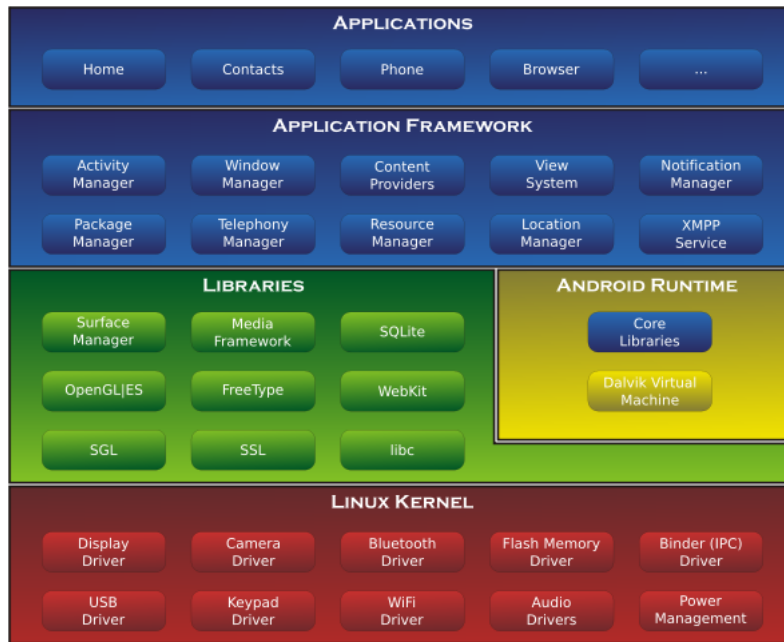
Figure 1.1: Android OS architecture. Image source: Wikipedia.
