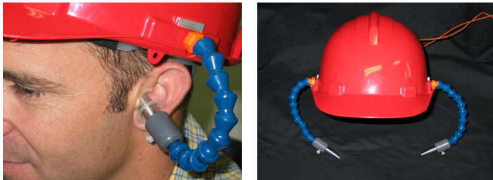
Figure 8-1. Ear probe inserted in participant's ear (left). Helmet and flexible arms holding the ear probes (right).
