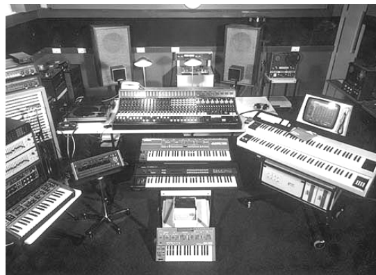
Figure 1: EMS Studio c.1982 (later, the Multichannel Studio). Chilton 24.8.2 desk (middle), Publison DHM89 digital delay/pitch shifter (bottom left), Fairlight CMI series II (right).
