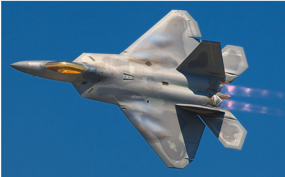
Figure 2.4: Mach Shock Diamonds formation of F-22A manoeuvring at high altitude (Flow Underexpanded )[4].
