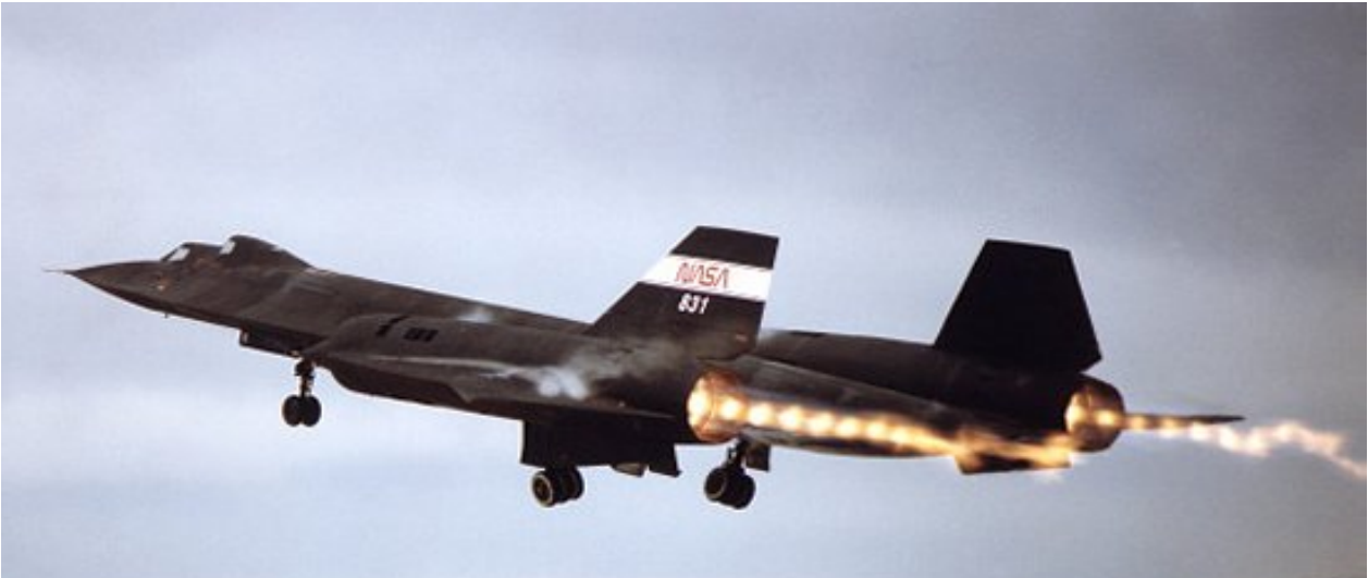
Figure 2.3: Mach Diamonds during take-off of SR 71 (Flow Overexpanded ) [1].
