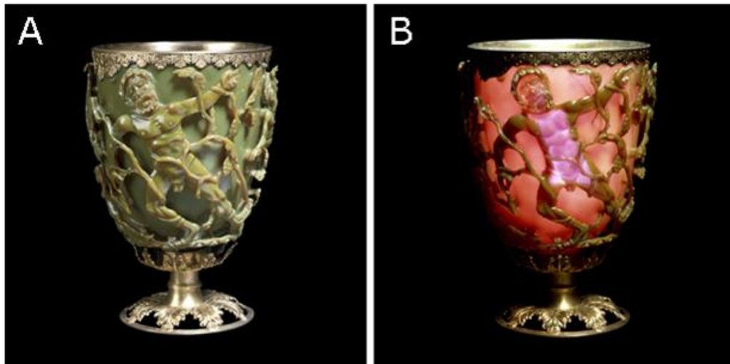
Figure 2: The Lycurgus cup demonstrating different optical effects depending on whether the light is reflected off the glass surface (A) or transmitted through the glass (B). Image adapted from http://www.guardian.co.uk/nanotechnology-world/nanotechnology-is-ancient-history
