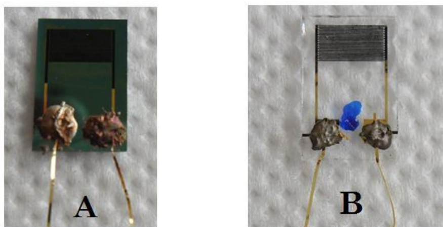
Figure 5.3. (A) A sensor based on nanostructured polythiophene deposited by two-electrodes cell, (B) A sensor based on polypyrrole nanowires deposited by a three-electrodes cell.
