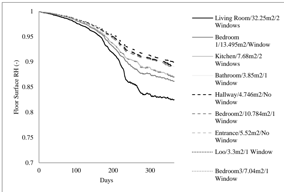
Figure 7. The drying of the surface of the floors in a bungalow using natural drying, for different rooms/ room footprint areas / and access to natural ventilation.
