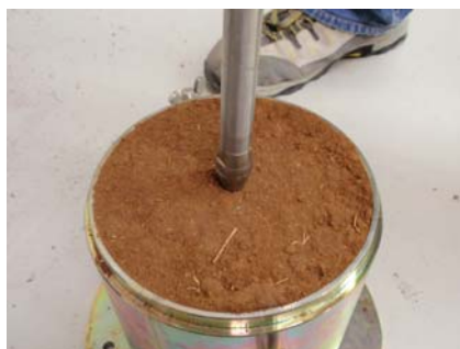
Fig. 1 DCP test in the CBR mould (M1) and in the 700 mm × 700 mm × 700 mm mould (M2).
