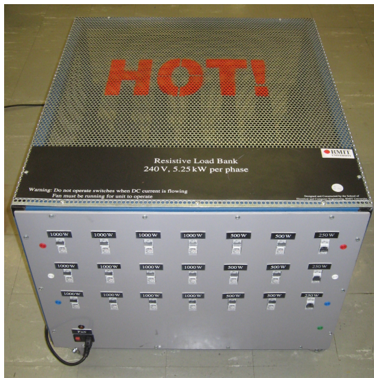
(a) Resistive Load Bank
