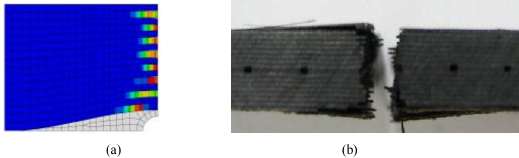
Figure 6: (a) FEA of fibre failures in the composite containing the 680 micron microvascular fibre aligned in the transverse direction. The colour coding shows the fibre fracture damage index. (b) Tensile failure of the same composite determined by experimental testing.
