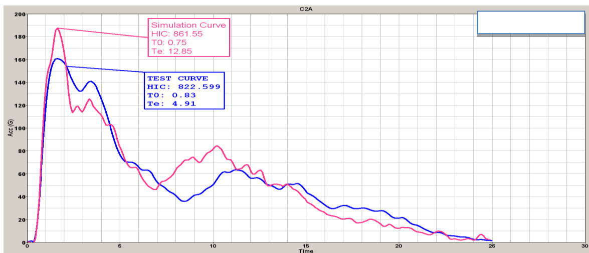
Figure 7.10: Correlation between ANCAP test and FE simulation
