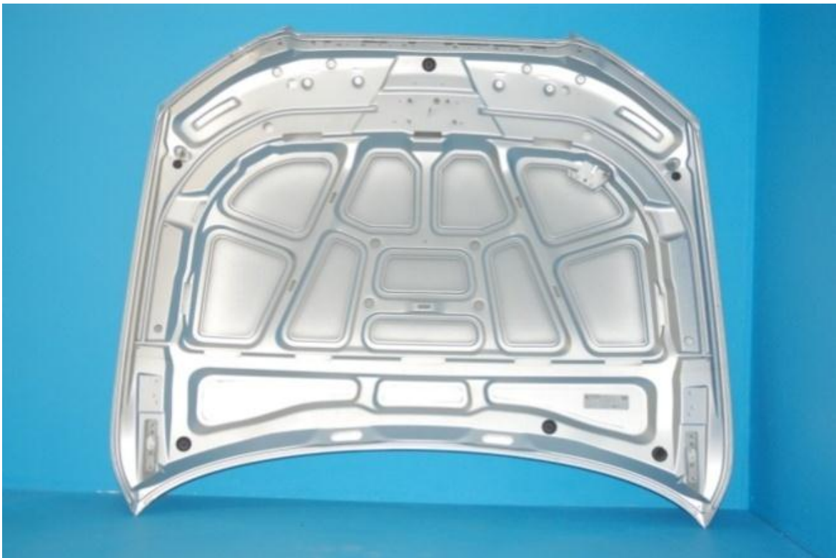
Figure 3.13: Skeleton structure for inner hood (A2Mac1 2010)
