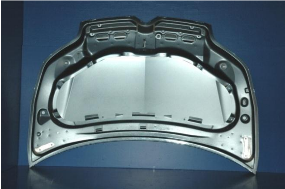
Figure 3.14: Cut-out structure for inner hood (A2Mac1 2010)
