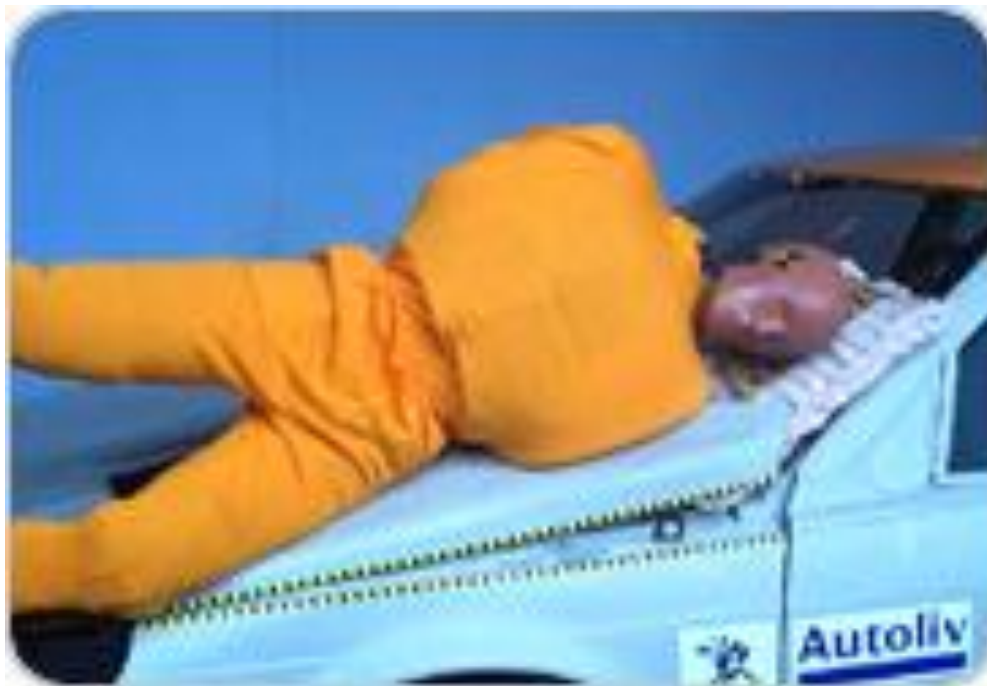
Figure 3.11: Airbag to cushion pedestrian impact on the A-pillar (Autoliv 2009)
