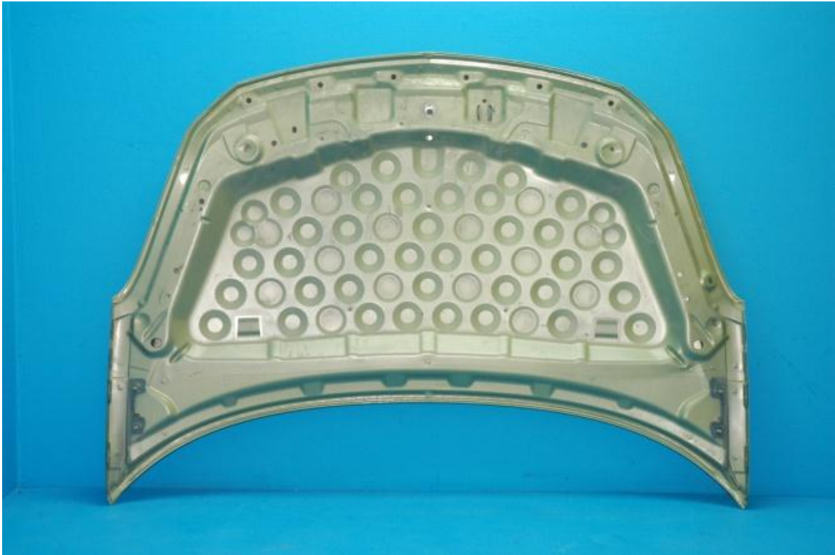
Figure 3.12: Multi-cone structure for inner hood (A2Mac1 2010)
