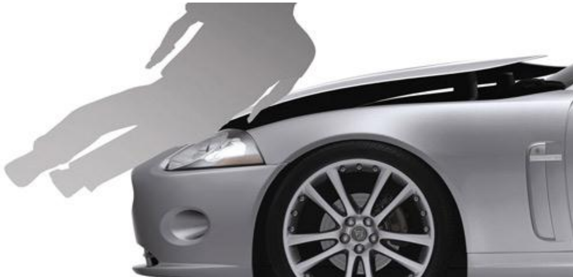
Figure 3.9: Active hood in a pedestrian impact scenario (Autoblog 2005)
