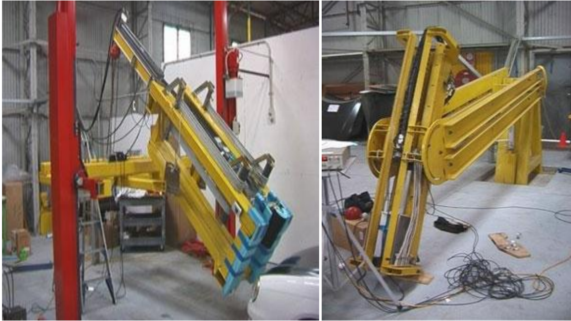
Figure 5.6: Leg impact and head impact test machines (Centre of automotive safety research 2007)
