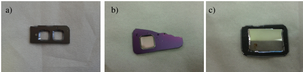
Figure 2.7: The final produce of the wet etching using different masks a) double circular mask b) square mask and c) rectangular
