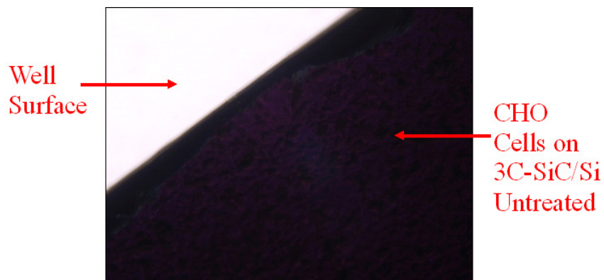
Figure 5.5: Optical micrograph of CHO cells cultured overnight on 3C-SiC/Si untreated at 20× magnifications.
