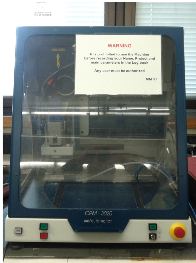
Figure B.1: isel CPM 3020 which was used to remove the 3C-SiC layer exposing the substrate for KOH wet etching of Si.
