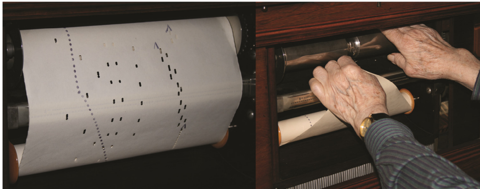
Figure 47. The punch holl role of a player piano as showed by Reg Richings at the ReStore, Ealing London.
