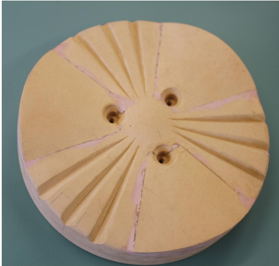
Figure 43: Hand carved hat block for vacuum forming
