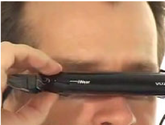
Figure 14. Typical Contemporary Lightweight LCD Video Eyewear
