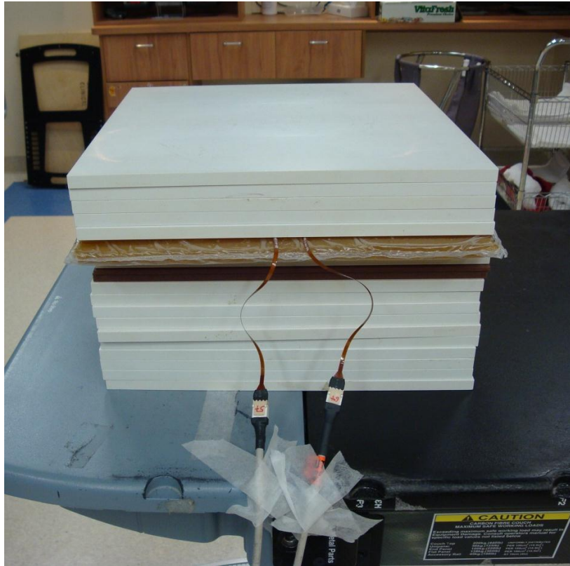
Figure 4.7 Photograph of the set up for the energy response measurements using the 6 MV and 18 MV linac.
