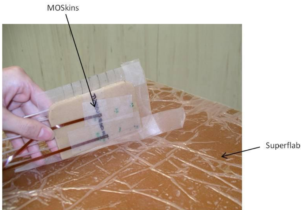
Figure 5.5 Photograph of two MOSkins taped to the underside of the IOBT applicator at measurement positions A1 and A7.
