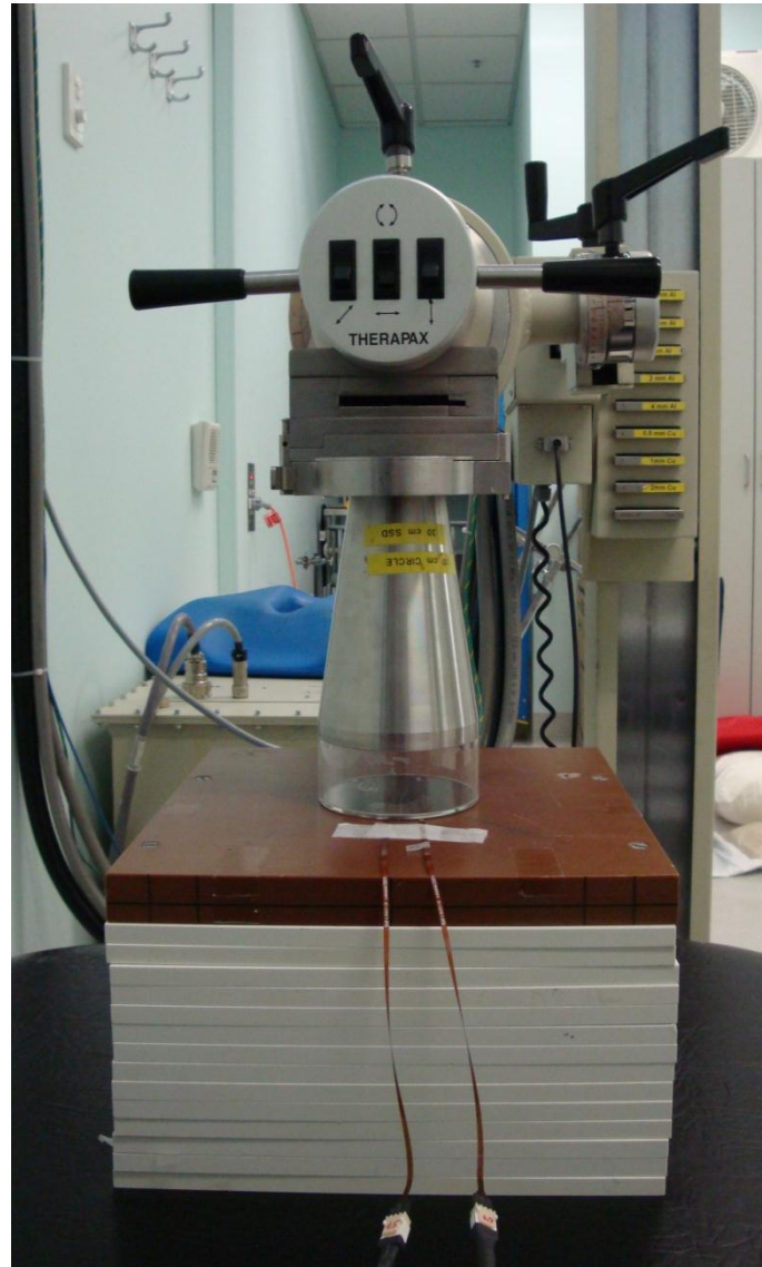
Figure 4.6 Photograph of the set up of the energy response measurements using the deep and superficial X-Ray unit.
