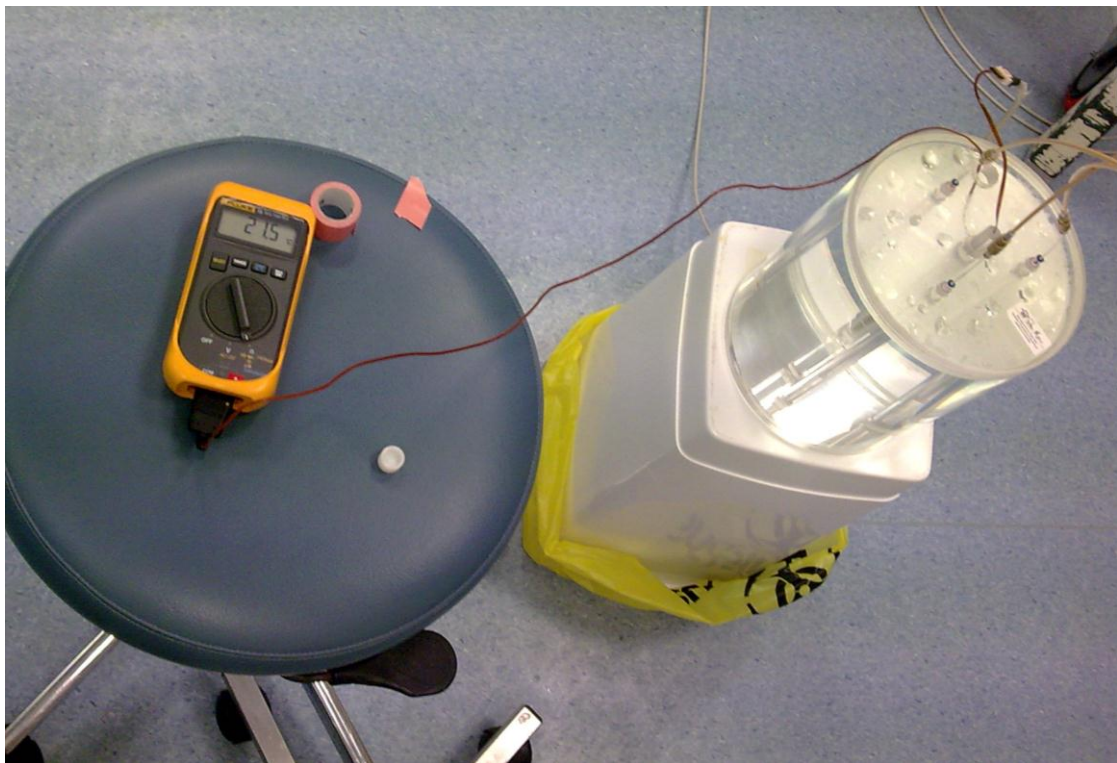
Figure 3.12 Photograph of the cylindrical PMMA water phantom with the digital thermometer inserted via the plug hole at the top.
