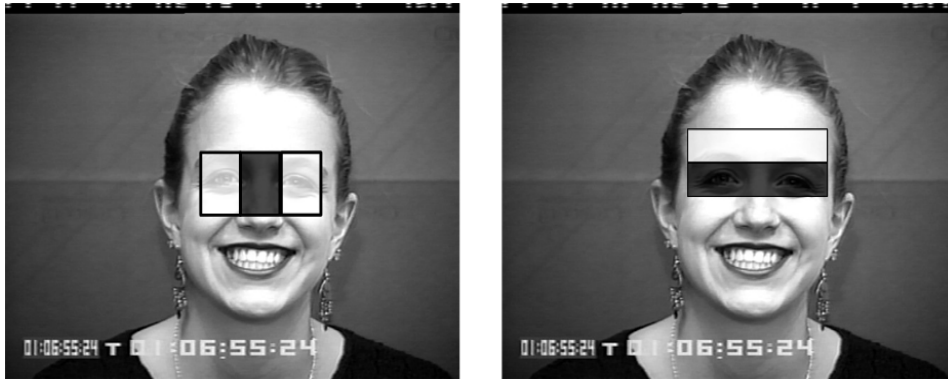
Figure 3.3: Two main rectangular Haar-like features for face detection
