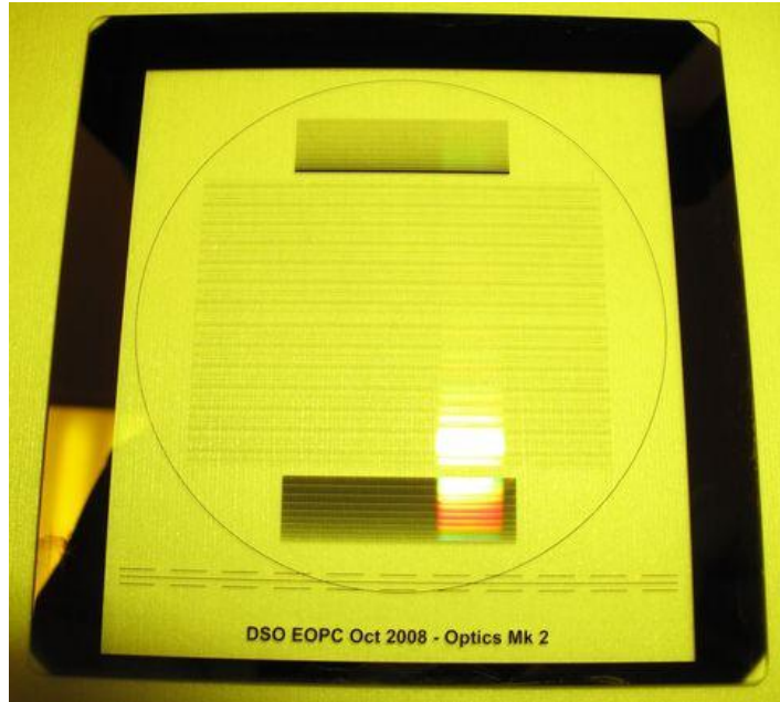
Figure 3.4: Photograph of waveguide mask used for fabrication.
