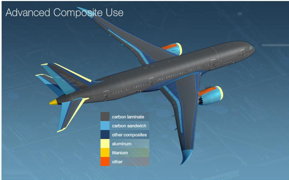
Figure 2.3 Advanced composite use in BOEING 787 commercial airplane (Courtesy: BOEING).
