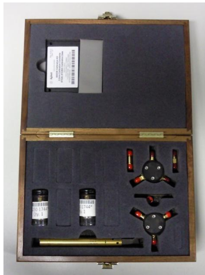
Figure 6.12 Calibration kit used for antenna measurement.
