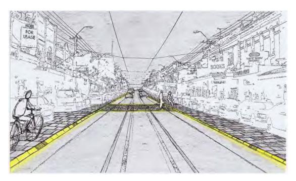
Fig. 5.10 – Paved and illuminated pedestrian crossings
