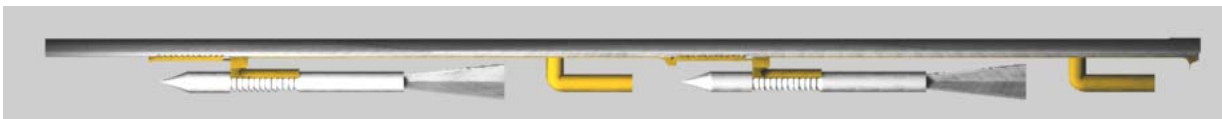
Figure 6.7: Segmented Sabot Design: Two Rounds located inside the Barrel (Quarter Model shown)
