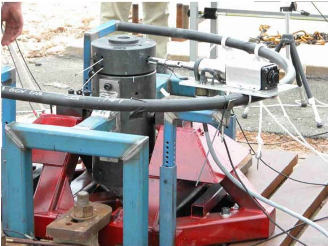
Figure 8.12: Test Rig Set-Up in Vertical Firing Position.
