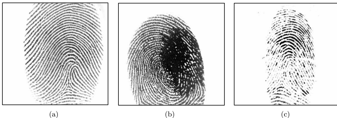
Figure 2.9: The fingerprint images (a) a high quality fingerprint (b) and (c) low quality fingerprints caused by noises, which result in inaccurate or missing some features (fingerprint images are taken from FVC2002 [61]).
