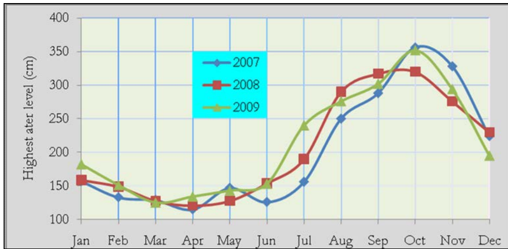
Figure 5.16a: The highest water level of the Hau River, measured at the Chau Doc hydro-meteorological station. Source: An Giang Statistical Bureau (2010)
