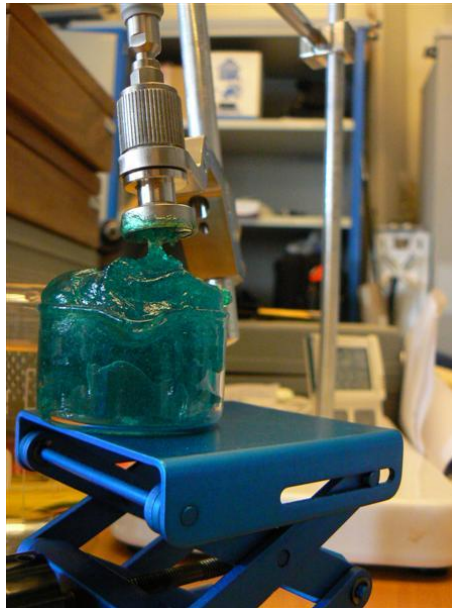
Figure 16: High concentration of gelling agent makes for a grainy texture; dielectric properties are difficult to measure. Food dye was added to differentiate tissues.
