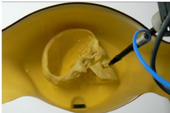
Figure 14: Initial tests using adult skull in flat part of SAM phantom at EMC Technologies, Melbourne, Australia
