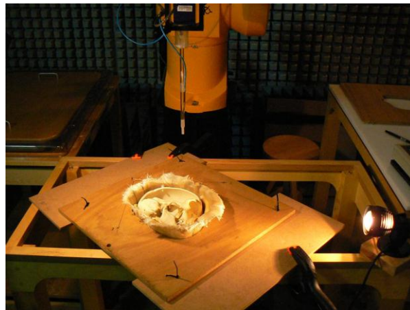
Figure 51: phantom and wooden frame with DASY4 system
