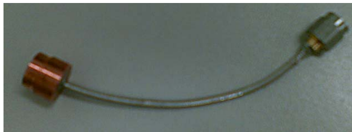
Figure 4.19 The fabricated balun for Antenna II
