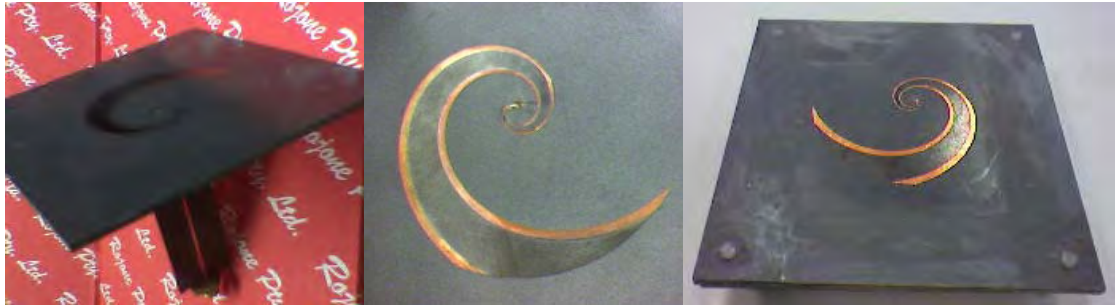
Figure 2.15 Three fabricated spirals with TFRL (a) Model X with 20nm TFRL (b) Model Y with 18nm TFRL (c) Model Z with 15nm TFRL
