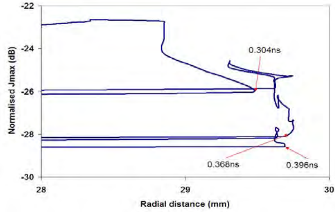
Figure 3.7 J_{\max} of Model B in free space vs. radial distance with higher resolution
