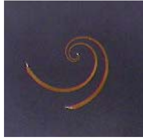
Figure 3.12 The single arm spiral with split loaded by one pair of resistors
