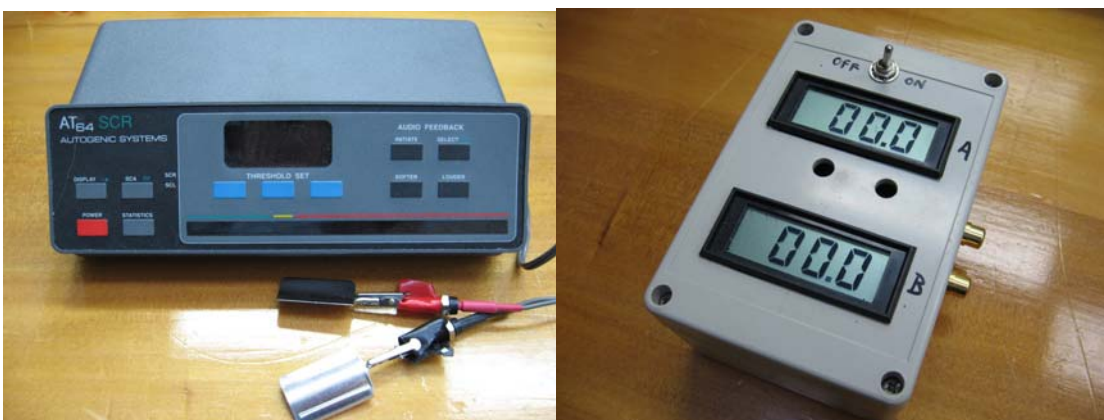
Figure 13 SCL/SCR meter used initially for GSR tests (left) and Pressure meter (right).
