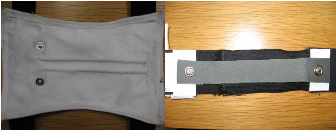
Figure 44. Strain sensors, CSIRO monofilament (left), PPY (right).
