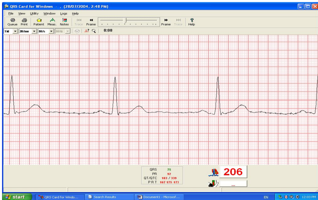
Figure 41. ECG signal as displayed on QRSCard, RA, LA AgNylon, RL, LL Stainless steel.
