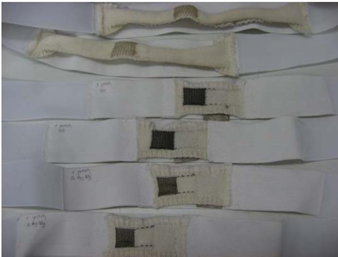
Figure 49. Pairs of fabric test electrodes sewn onto bands for initial single subject tests, top AgCu, mid SS, bottom AgN.
