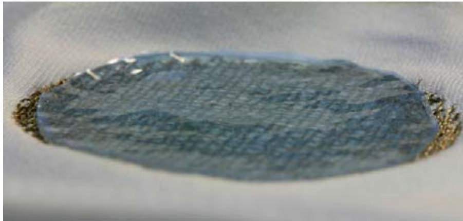
Figure 7. Embroidered circular electrode with solid gel covering for better skin contact (redrawn from [94])
