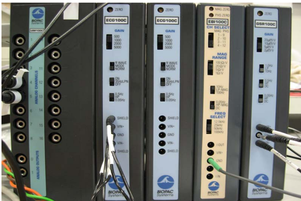
Figure 14 Biopac system hardware used for GSR and ECG tests.
