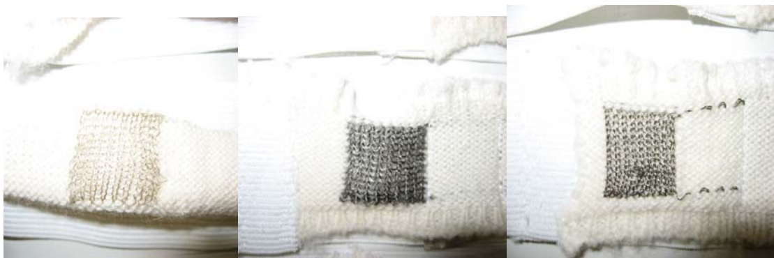
Figure 17. Knitted electrodes on loose knitted band (used for first single trials), left to right; Silver Copper, Stainless steel and Silver Nylon.
