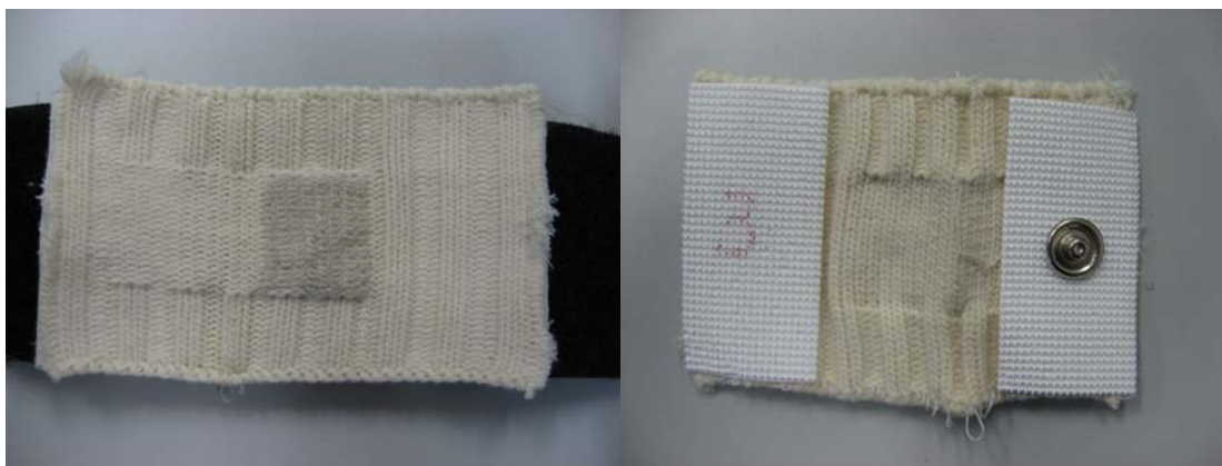
Figure 21. Detachable fabric electrodes (AgCu(s) example), front and rear views
