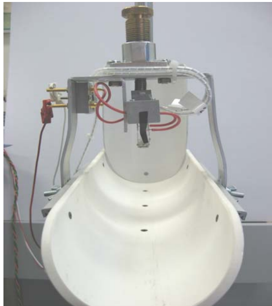
Figure 26. Final pressure electrode test rig used for GSR tests on subject forearm.
