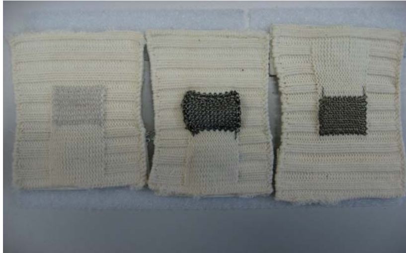
Figure 18. Actual knitted removable electrode assemblies, used for multiple trials, left to right; Silver copper, Stainless steel and Silver Nylon.
