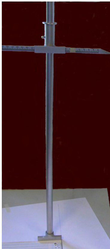
Figure 6.1. Height measuring gauge for toile and pattern balance
