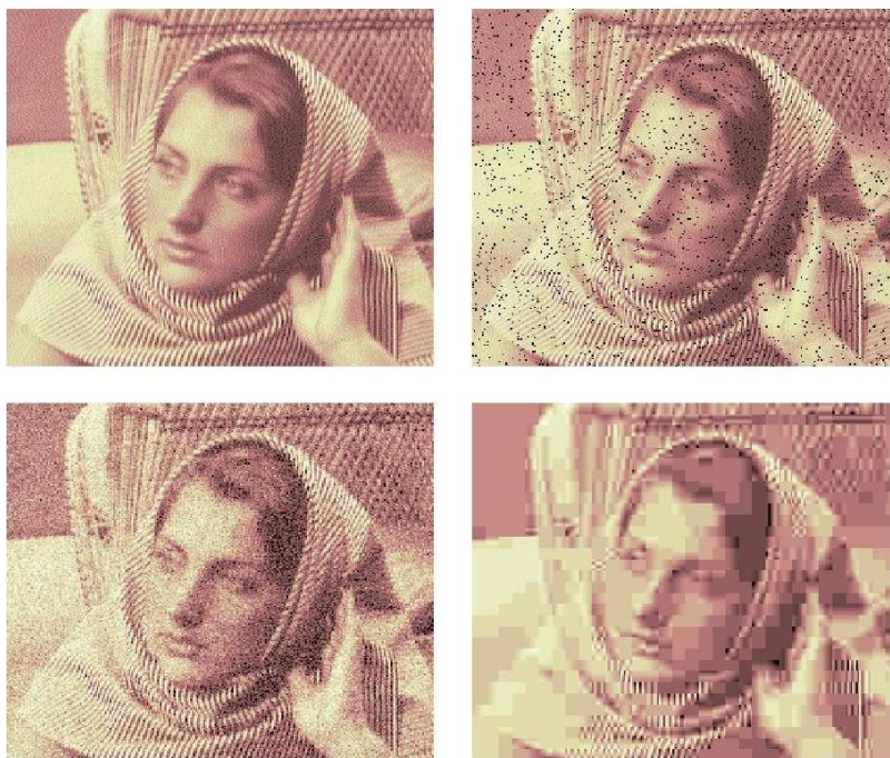
Figure 4.2: Clockwise: Original image, image corrupted with impulsive noise, lossy JPEG compressed image and image corrupted with AWGN.
