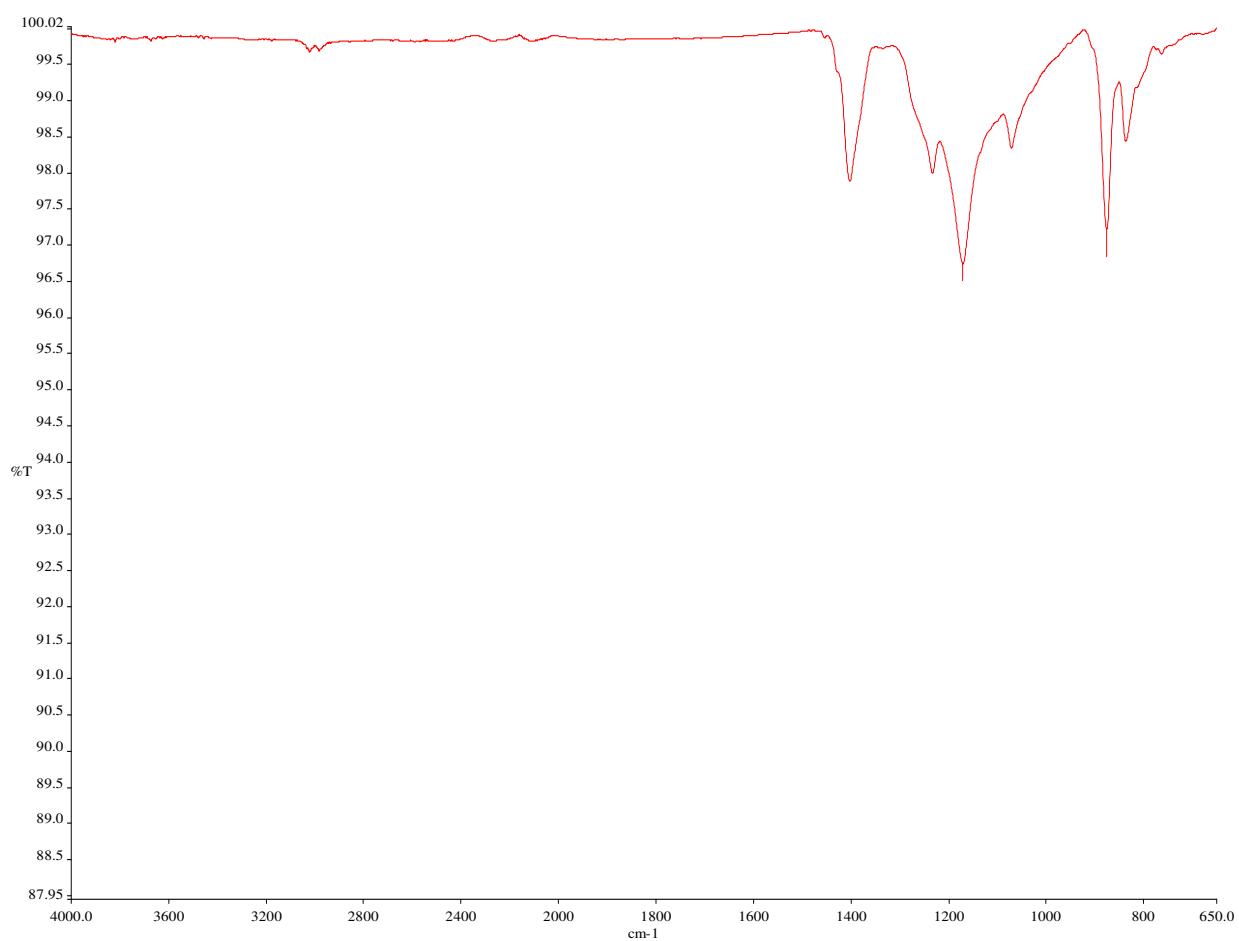
Figure 3-9: A typical plot FTIR spectrum for poly(vinylidene fluoride)-hexafluoropropylene
