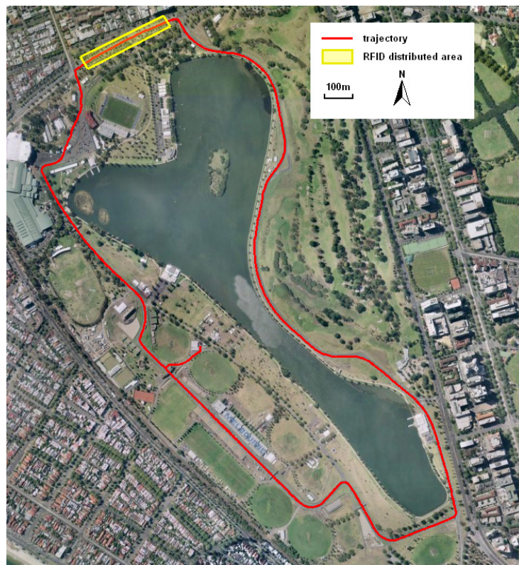
Figure 6.2 The experimental site and the trajectory for evaluating the iterated reduced SPKF for the GPS/RFID integrated seamless positioning technique
