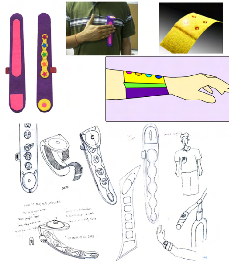
Image 74 Produced by Zhu Yu Lin The device can be worn on the cyclist's wrist or put in their chest pocket, depending on which way they could better feel the vibration signals.
