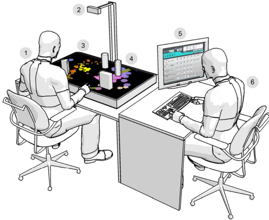
Figure 5: Illustration of Elements prototype. Image key - 1) Patient; 2) Computer vision camera and mount; 3) Patient display; 4) TUIs; 5) Therapist display; 6) Therapist administrator
