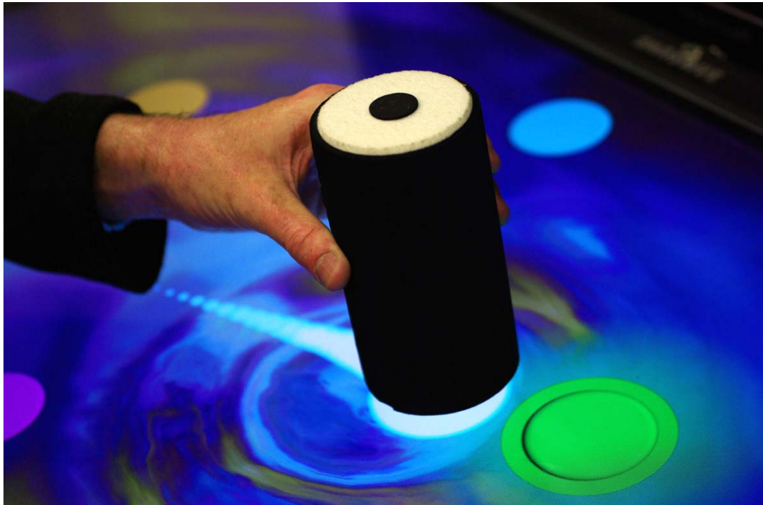
Figure 16: Examples of audiovisual feedback - Water Ripple, Trail at the base of a prototype TUI, and Target aura
