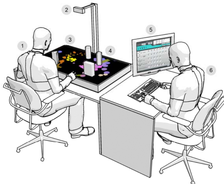
Figure 1: Illustration of Elements prototype. Image key - 1) Patient; 2) Computer camera and mount; 3) Patient display; 4) TUIs; 5) Therapist display; 6) Therapist administrator
