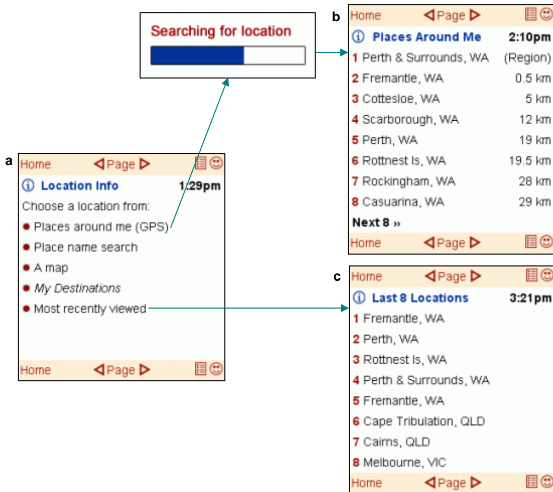
Figure 9.3 (a) The 'location info' search menu; (b) searching for a location using automated (A-GPS) input; and (c) searching within a list of recently viewed locations.
