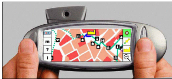
Figure 3.8 A 'detail' map within the Lol@ interface showing a landmark silhouette, category map symbols and a tour route (Gartner & Uhlirz 2001).
