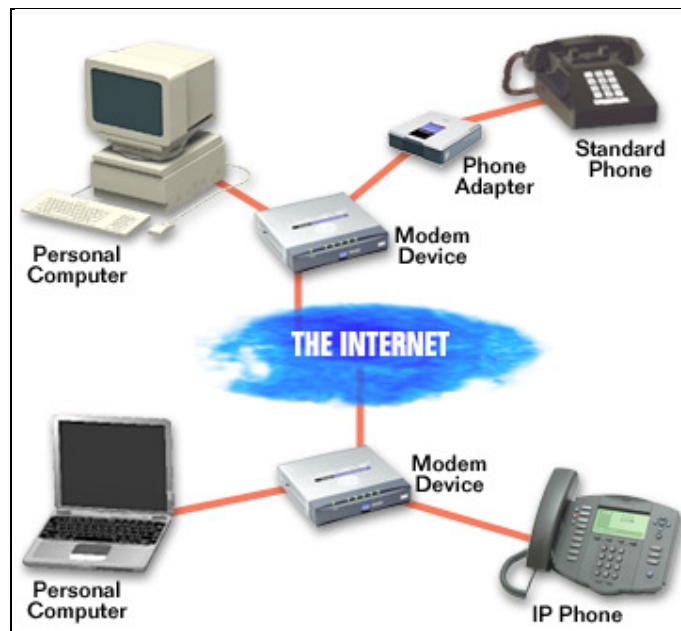
Figure 2: VoIP Connection Methods
