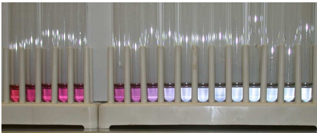
Figure 3.9. Image of the critical flocculation experiment (CFC) experiment of 50 nm gold nanoparticle conjugated with OMP 85 protein. Similar experiment was performed with anti-OMP85 antibody conjugated 50 nm gold nanoparticles. Both were stable up to a final concentration of 0.512 M NaCl.
