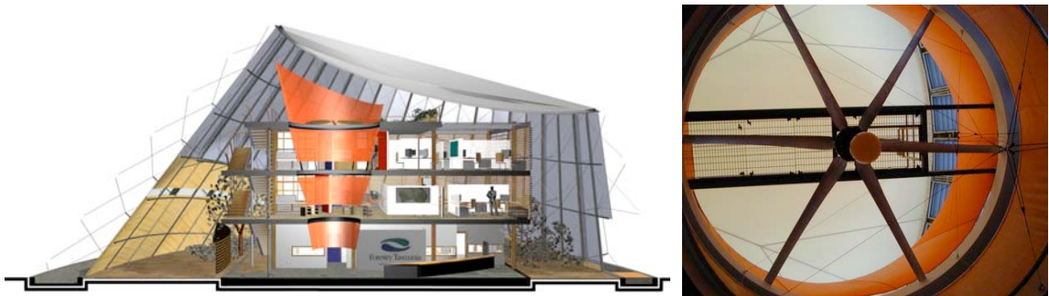
Figures 22/23: Forestry EcoCentre: cross-section and view of interior looking up the cone at the horizontal fan.
