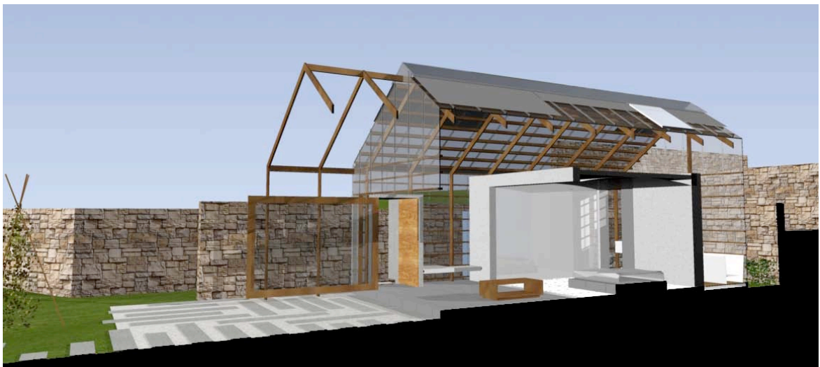
Figure 36: View towards the dry stone rubble enclosing walls, which surround each pavilion with a cutaway cross section showing (right to left), and 'outdoor' sitting area, a central sleeping cell, and at rear the private bathroom,
