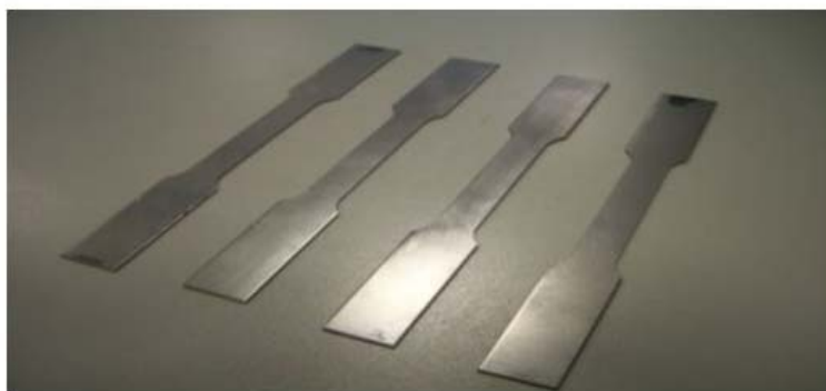
(b) Prepared tensile test specimens
