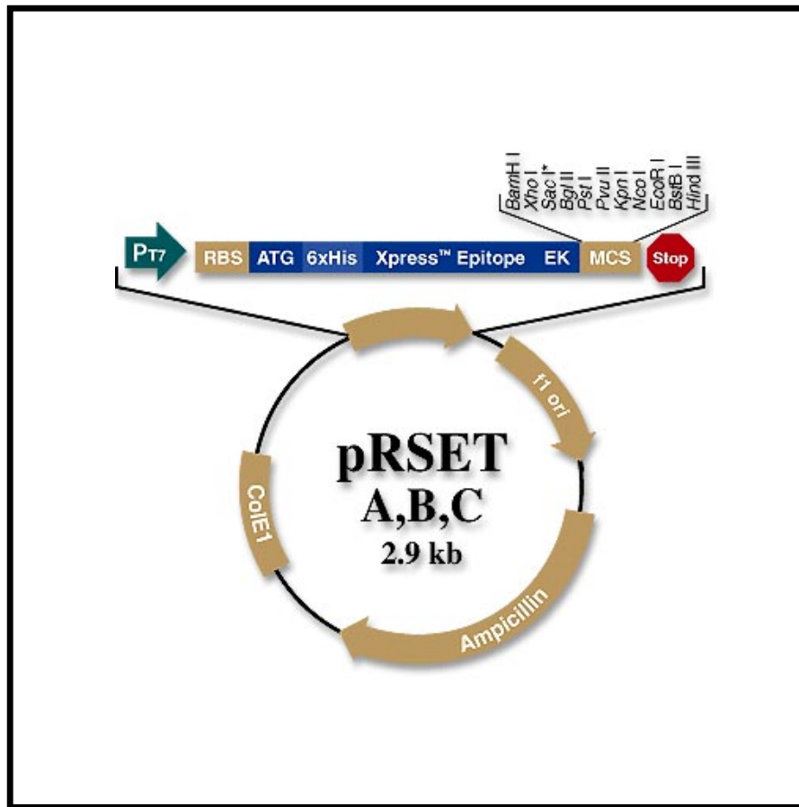
Figure 6.3. Physical map of the plasmid pRSET, displaying the major plasmid features (www.Invitrogen.com). These include the T7 Promoter gene ( P_{T7} ), the 6 x Histidine tag (6 x His), the Ribosome binding site (RBS), the Multiple cloning site (MCS), the E. coli origin of replication (ColE1), the Phage 1 origin of replication (f1 ori) and the ampicillin resistance gene.
