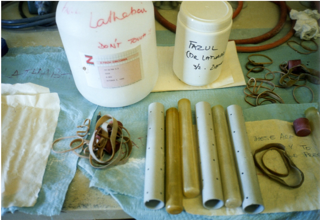
Figure 3.13: Flexible Elastomeric Mould (Size of mould 150mm length diameter 30mm)
