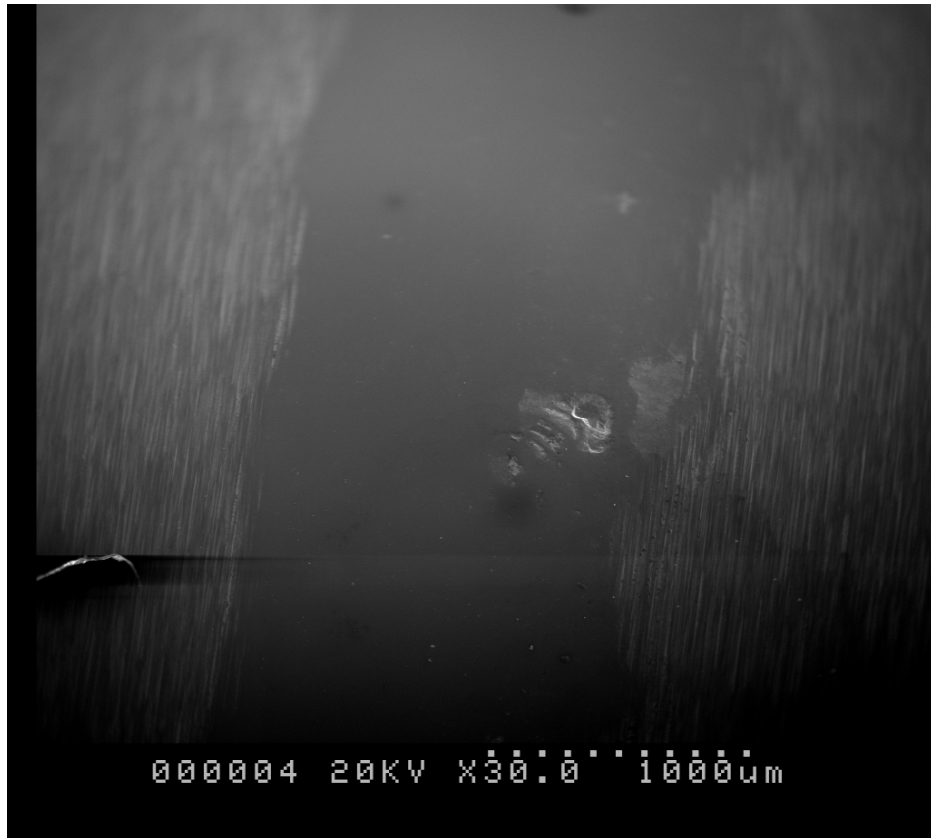
Figure 4.70 Sample 1, 330 min, 790N load. Highly polished surface with Fatigue Spallation.
