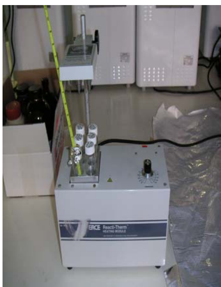
Figure 3.1: Photograph of the heating block used in the derivatising procedure of nitrofuran metabolites
