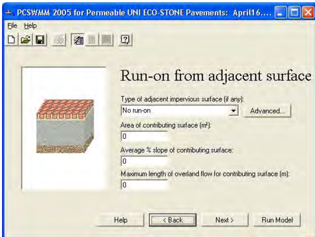
Figure 5.6 Interface for run-on from adjacent surface
