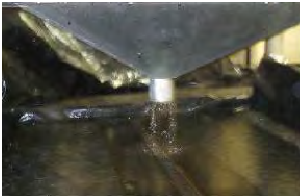
Figure 3.4 The funnel attached to collect the infiltrated water (Zhang, 2006)
