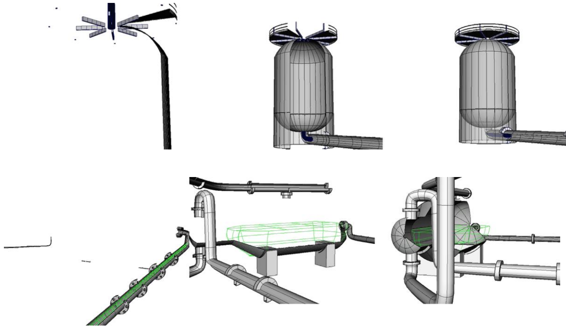
Figure 52 (top) Mercury Removal Unit and (bottom) Propane Heat Exchanger “drawn on” by animating their construction histories, 2006
