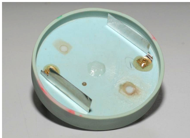
Figure 3-1 Electrodes fixed on a polymer substrate. It is a part of the electrical cell for EIS measurements.
