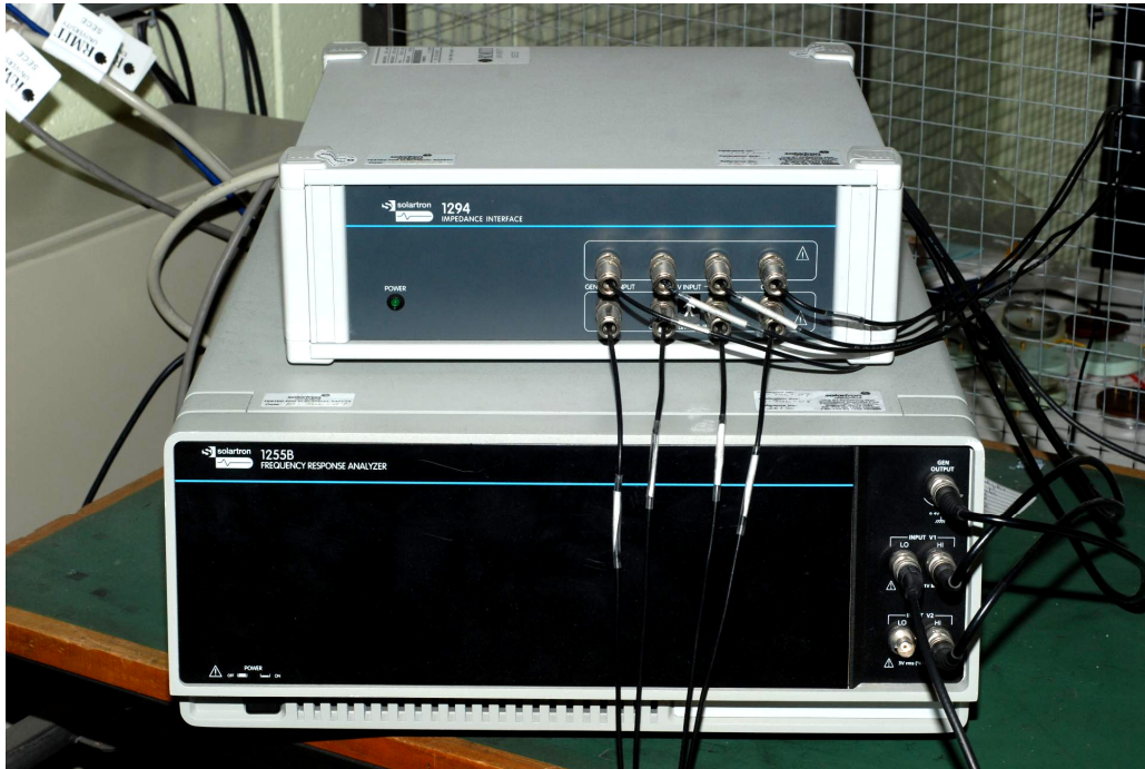
Figure 3-2 Solartron ® 1260A Impedance/Gain-phase Analyser and Solartron ® 1294 bio-impedance interface used in EIS measurements.
