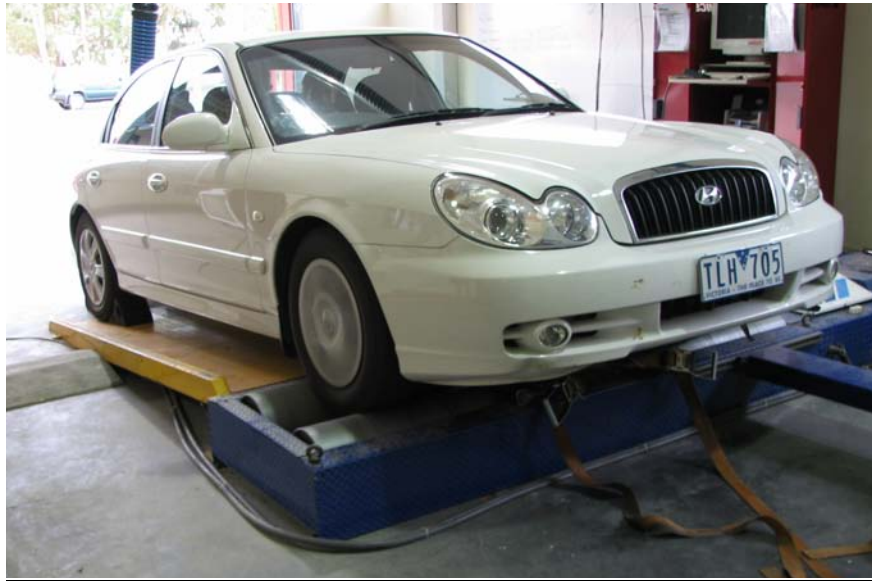
Figure 2.6: Hyundai Sonata testing vehicle was mounted on the chassis dynamometer.
