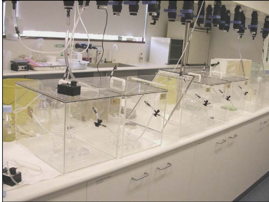
Figure 4.2 Experimental setup of five controlled atmosphere chambers, each set to a different oxygen-atmosphere concentration (and thus dissolved oxygen level).
