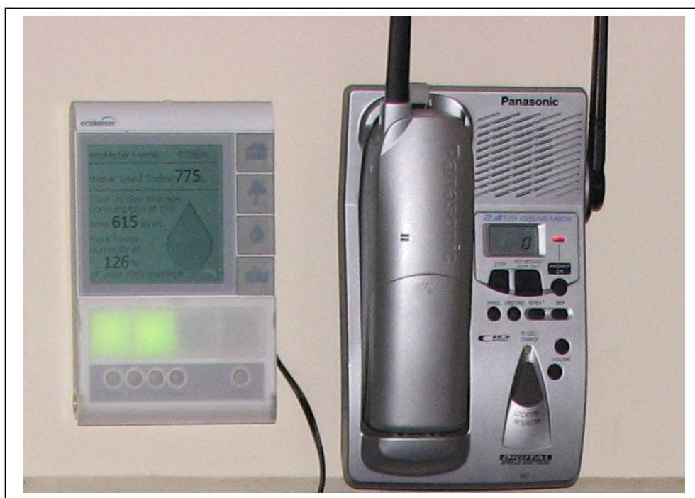
Figure 7.2: Green 'traffic lights' and consumption data displayed on an ecoMeter IHD
