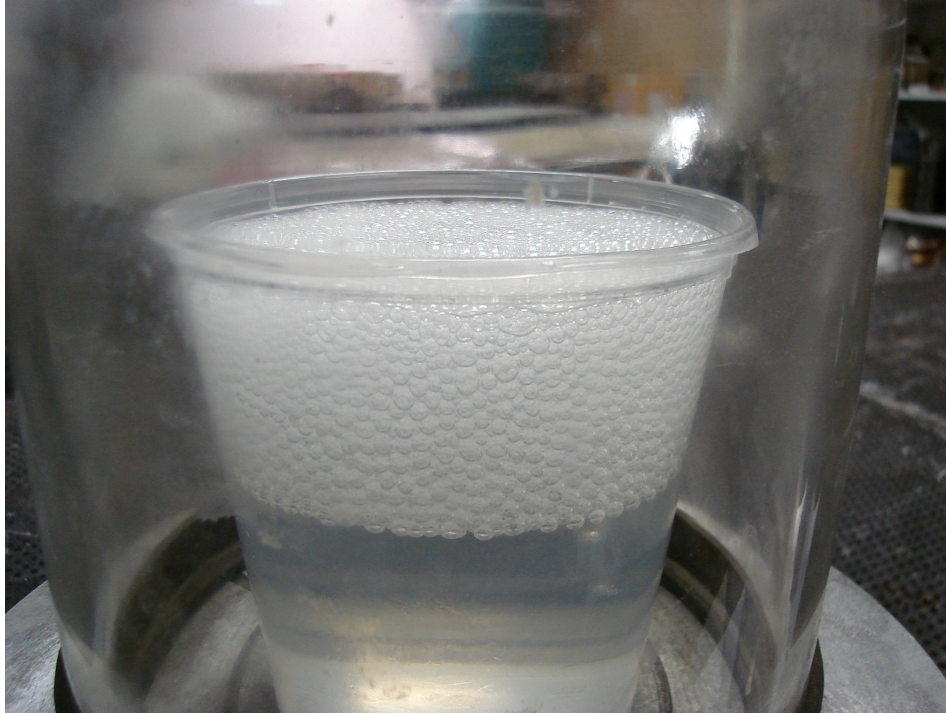
Fig. 5.4 The mixed silicone and curing agent are exposed to a vacuum to remove air bubbles and dissolved air
