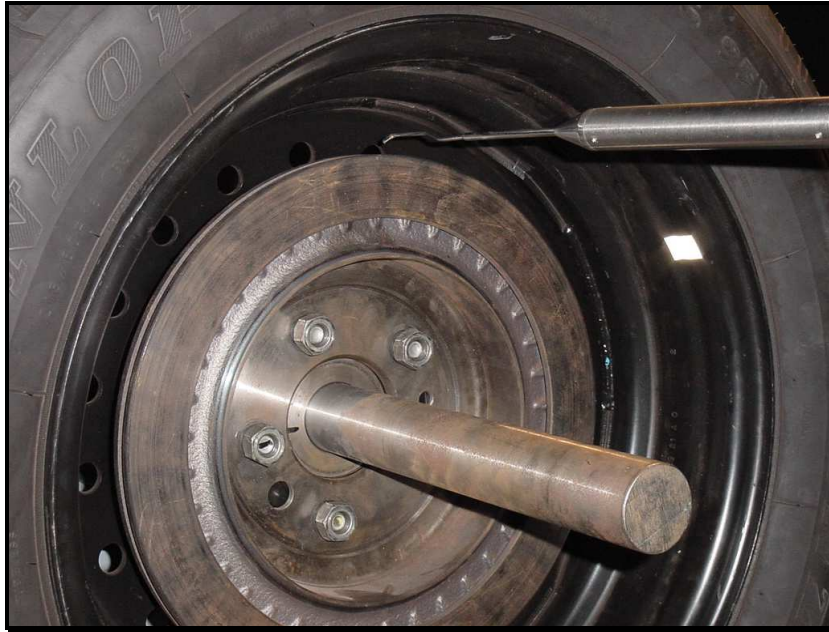
Figure 4.4.10 Airflow Measurements with Wheel in Place
