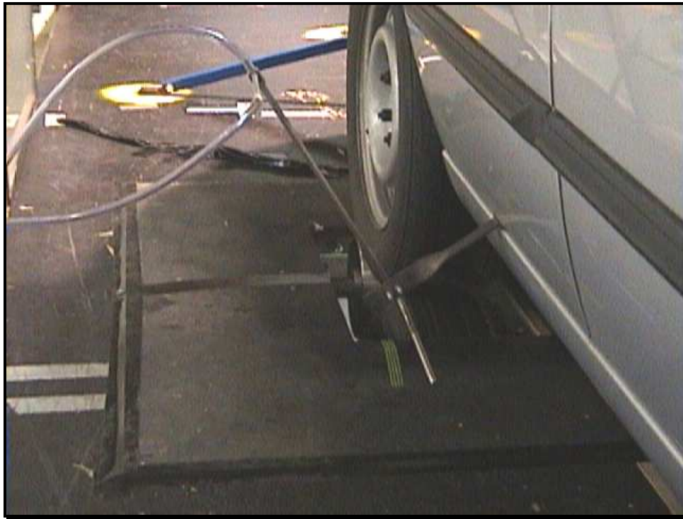
Figure 5.2.1 Local Velocity Measurement Using a Pitot Static Tube
