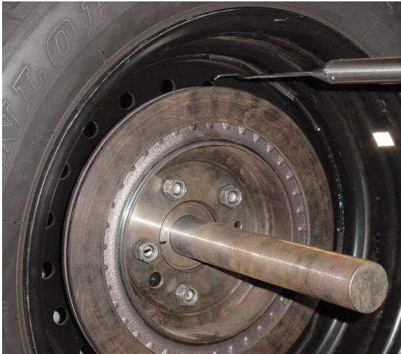
Figure 9 Airflow Measurements with Wheel in Place
