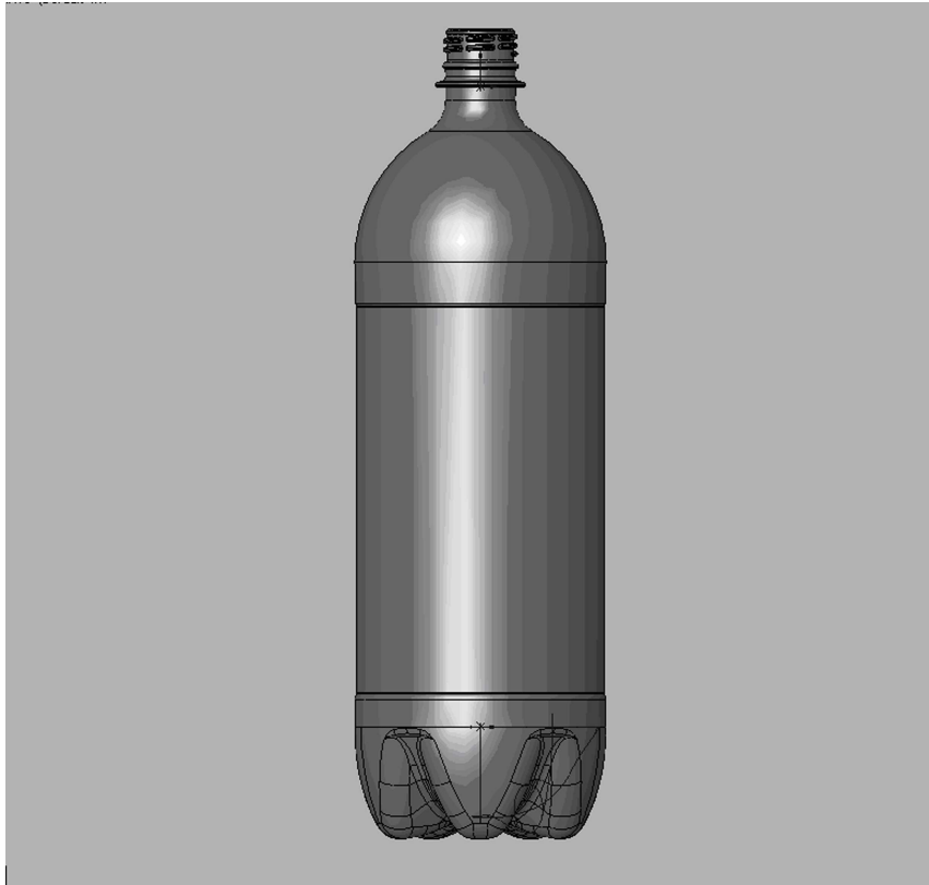
Fig.3-2. The CATIA drawing of the standard (current) PET bottle
