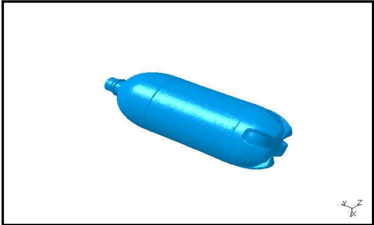
Fig.A-2. Deformed mesh on the bottle under the internal pressure of 0.4 MPa.
