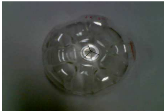
Fig.5-10. ESC at the bottom of the bottle with optimum base
