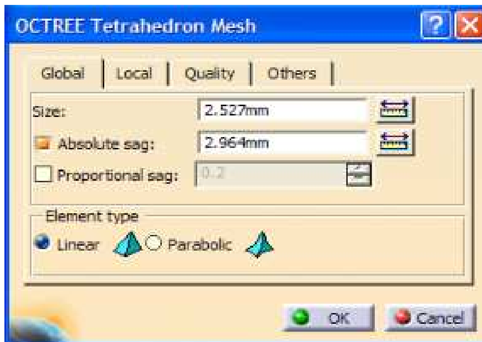
Fig.3-14. The mesh size used in the stress analysis
